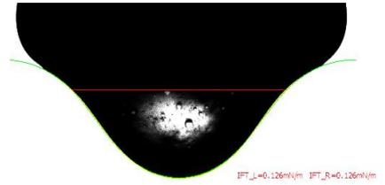
1. Contact angle measurement: The drop formed under high pressure is usually shaped into an approximate ellipsoid in 3D due to its gravity, hence we adopt Young-Laplace equation fitting technology (ADSA™) to fit its shape in 2D, and then calculate its contact angle between liquid drop and solid under gas or fluid surroundings.
