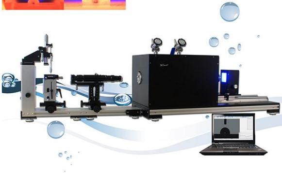
SL200HT series is a drop shape analysis based surface chemical analytical system for extreme conditions such as temperature of 2000°C, specializing in measuring surface tension and contact angle under ultra-high temperature, applied in research of mineral, metallurgy, ceramic, enamel, welding, semi-conductor, glass, alloy and coal and more. The super high temperature furnace,
