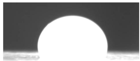
2. Surface tension measurement for melt under high temperature: For melted sample in high temperature, its surface chemical properties can be characterized by its drop shape profile; hence we here analyze it using Young-Laplace equation fitting method (ADSA™) via sessile drop method; melt volume and surface tension of melt can be calculated then.
